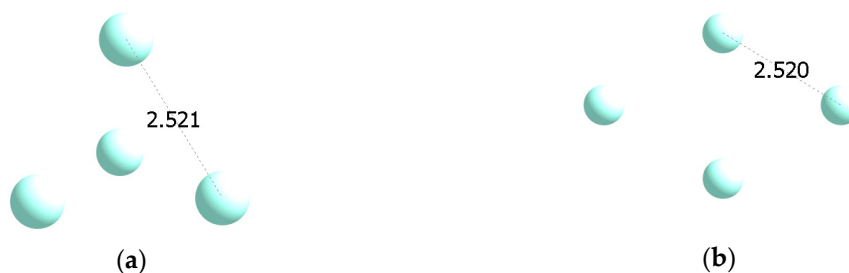
Figure 1. Tetrahedral (a) and rhombus (b) structures of \text{Co}_4 cluster; key distances are given in \text{\AA} .
