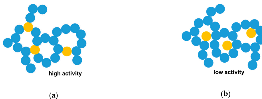
Figure 14. Schemes showing titania aerogels (blue) with gold NPs (yellow dots): (a) incorporated inside the titania network (3D Au–TiO 2 ); and (b) deposited on the surface of titania aerogels (Au/TiO 2 ); drawn based on references [165,166].
