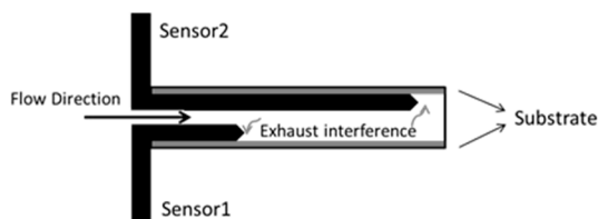
Figure 8. Layout of the thermocouples in the axial direction.
