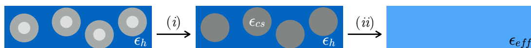
Figure 9. Procedure to reduce a system consisting on a composite core-shell type inclusion into a homogeneous slab.
