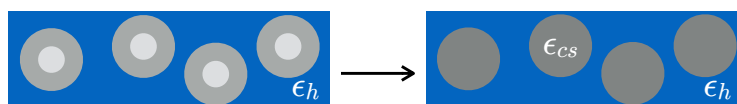
Figure 1. Scheme of the effective medium problem of composite with spherical core-shell type inclusions: the system formed by a composite with core-shell inclusions can be reduced to that of a composite with homogeneous spheres with effective dielectric function \epsilon_{cs} . The value of \epsilon_{cs} is obtained by applying an effective medium theory on the core-shell inclusion.
