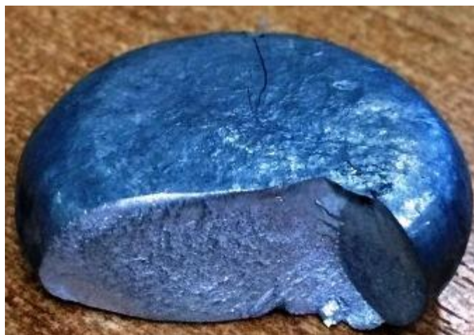
Figure 4. Macrostructure of master alloy 25Mg–50Zn–25Nd.
