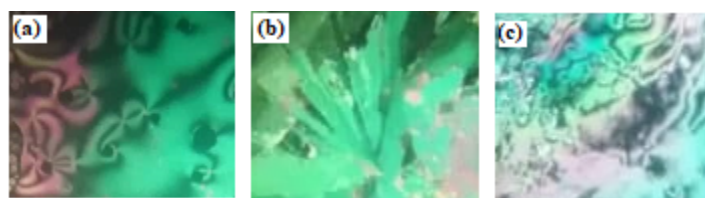
Figure S4. POM textures of binary mixtures upon heating (a) N phase of 60 mol% Ia for system Ic/Id at 112 °C; (b) SmA phase of 60 mol% Ia for system Ia/Ib at 84 °C ;(c) N phase of 60 mol% Ia for system Ia/Ib at 101 °C.
