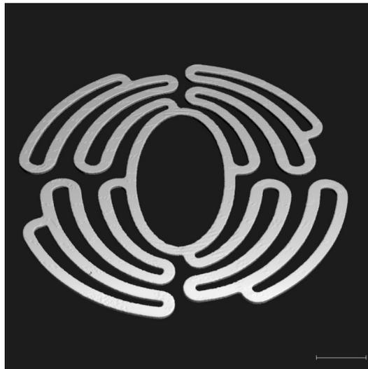
**Figure 2.** Reconstruction of the  $\mu$ -CT (Micro Computertomography) data of a magnesium scaffold prior to implantation. Bar indicates 5 mm.
