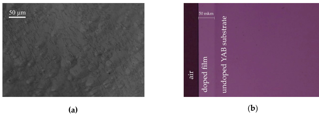
Figure 9. 50 \mu m thick as-grown (Er,Yb):YAB layer (a) and polarized optical image of the polished cross-section of the (Er,Yb):YAB layer on the YAB substrate (b).
