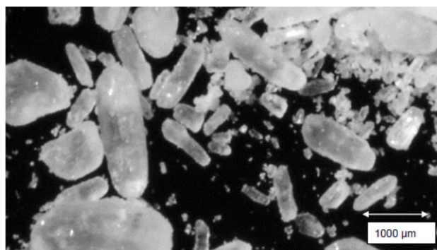
Figure 2. Optical characterization of commercial market product (broad crystal size distribution and elongated crystal shape).
