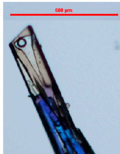
Figure 11. Photograph obtained by using polarized light microscopy showing the angle disruption in the conical shape fluid inclusion.
