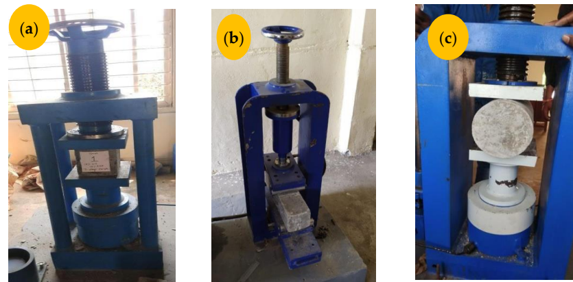
Figure 3. Hardened Concrete tests: (a) Compressive strength test, (b) Flexural strength test and (c) Split tensile strength test.
