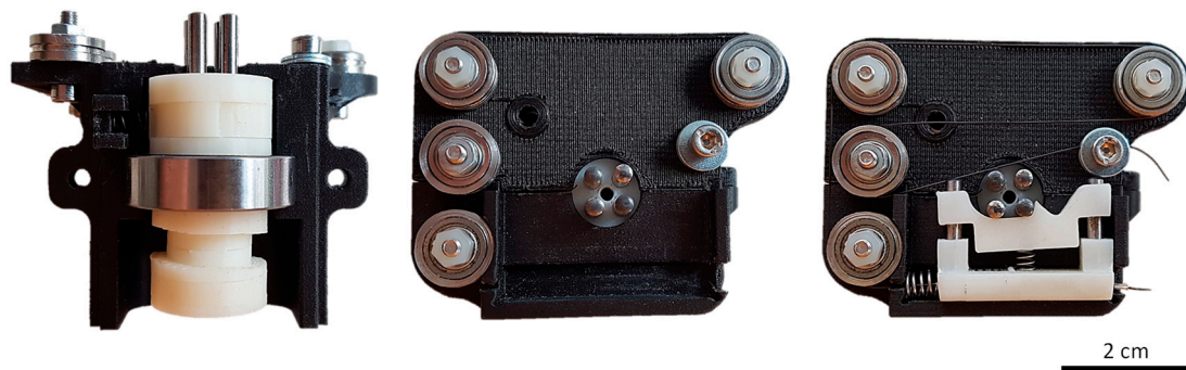
Figure 13. Assembly steps of the additive manufactured prototype.
