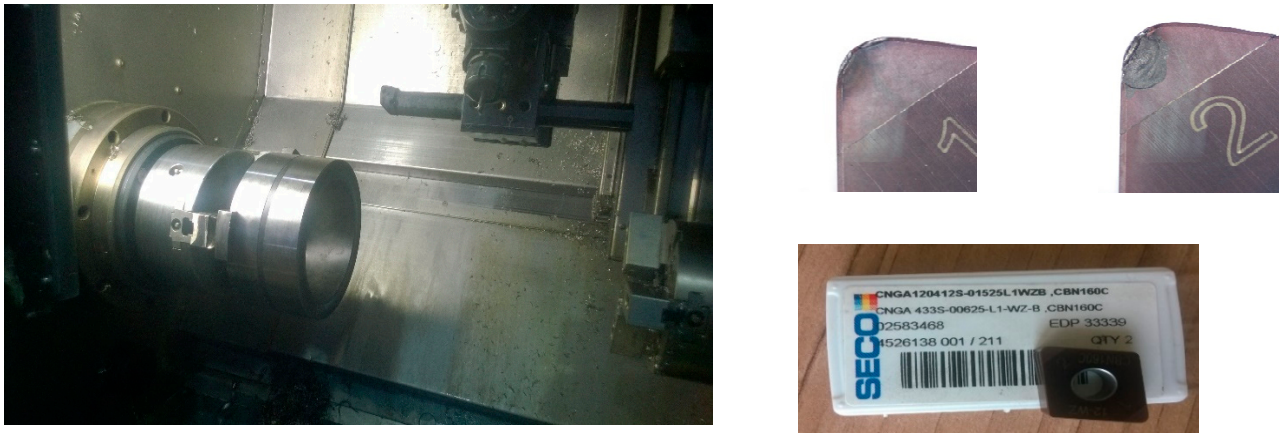
Figure 1. The machine SP280 SY workspace and details of cutting edge No.1 and No.2 inserts from cubic boron nitride (CBN).
