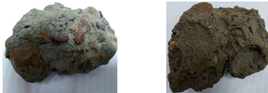
Figure 2. Original rough surfaces of the RCAs.
