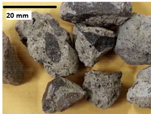
Figure 23. A low magnification image showing adhered cement in a RAC [87]. Reprinted with permission from Elsevier [87].
