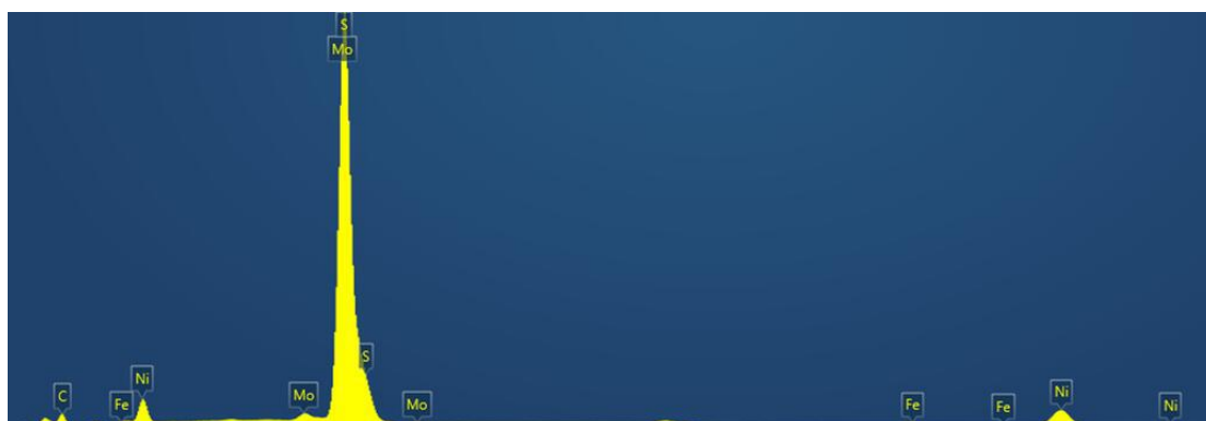
Figure S4. EDX analysis images of the Fe, C-MoS 2 /Ni 3 S 2 -450.
