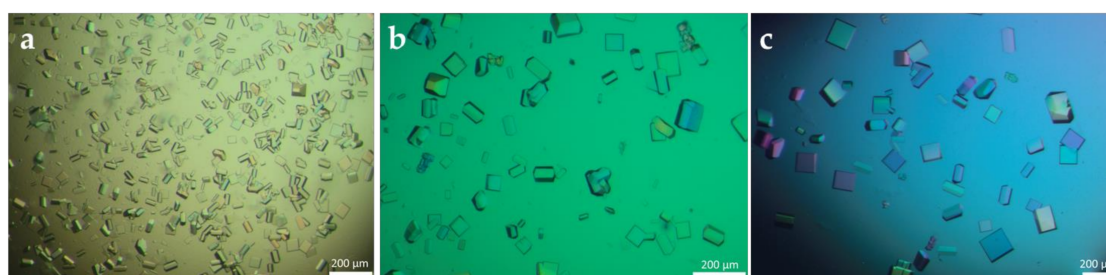
Figure 2. FJAT-PGA crystals formed under addition of seeds. Crystals were grown in droplets consisting of 4 \mu\text{L} FJAT-PGA solution (10 mg/mL), 4 \mu\text{L} FJAT-PGA crystallization buffer (8% ( w/v ) PEG 8000 in 100 mM HEPES pH 7.5) and 2 \mu\text{L} of appropriate FJAT-PGA crystal seed suspension (a–c). Seeds were obtained by crushing previously grown FJAT-PGA crystals. (a) No dilution of prepared seeds, (b) addition of a 10-fold diluted seed suspension and (c) addition of a 100-fold diluted seed suspension. The white line represents the scale.
