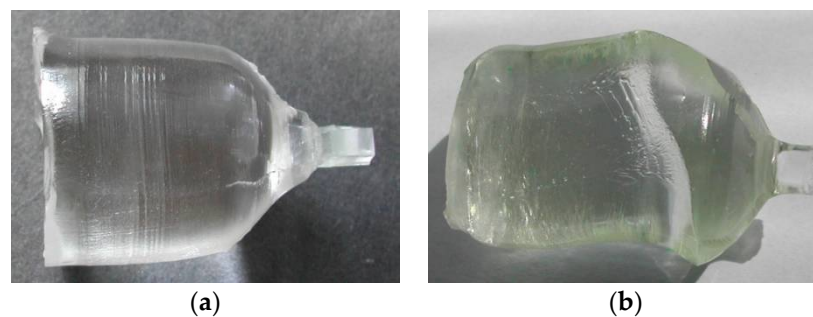
Figure 1. 1 mol% (a) and 5 mol% (b) Dy doped Li 6 Y(BO 3 ) 3 single crystals grown by the Czochralski method. The cylindrical part is 30 mm long and 25 mm in diameter.
