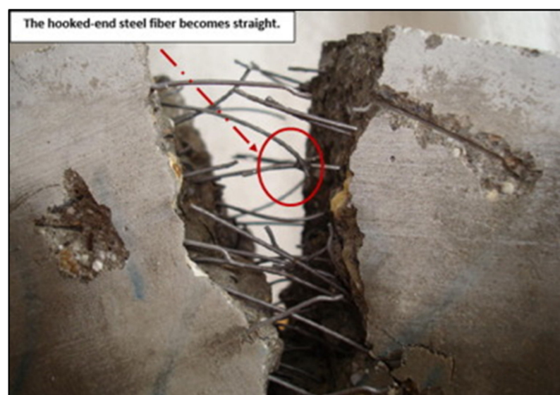
Figure 1. Concrete reinforced with steel and polypropylene fibers, reprinted with permission from Afroughsabet, Vahid., Ozbakkaloglu, and Togay. Elsevier.
