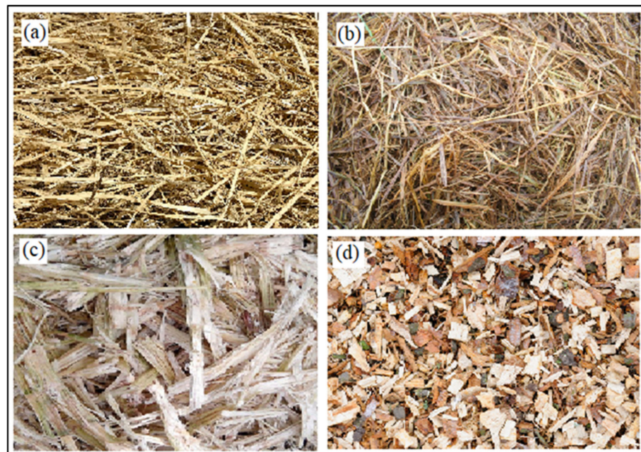
Figure 9. Raw forms of (a) wheat straw, (b) rice straw, (c) sugarcane bagasse, and (d) forest residues.
