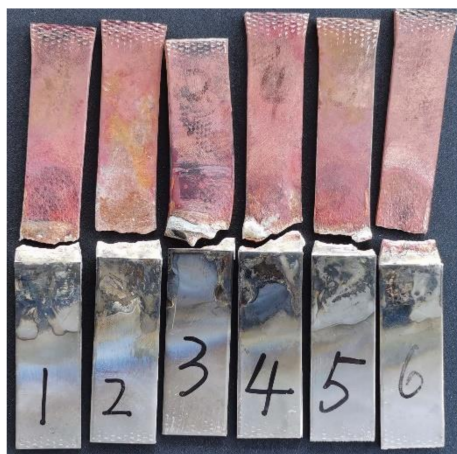
Figure 9. Copper/304 stainless steel lap tests.
