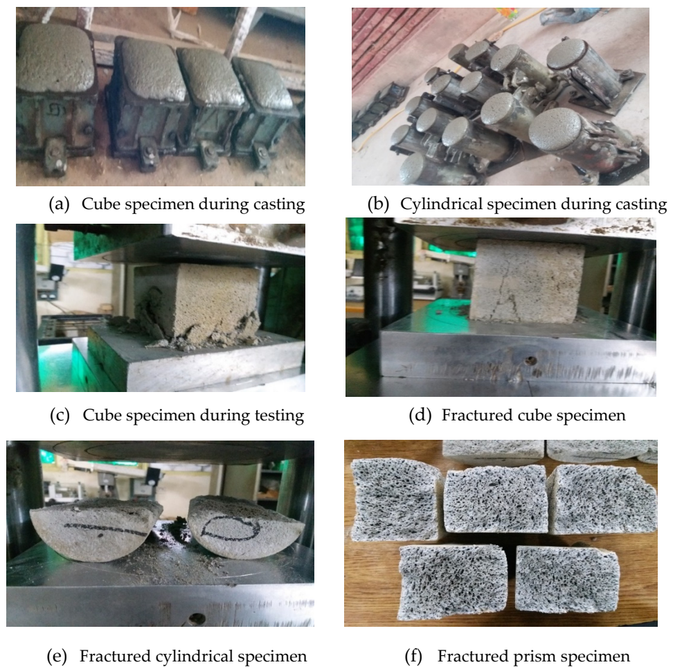
Figure 5. Fabricated and fracture images of all specimens (a–f).
