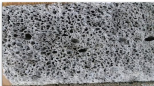
(c) Cross-section of cylinder specimen
