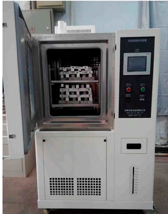
Figure 7. High- and low-temperature hygrothermal cycle experimental chamber.
