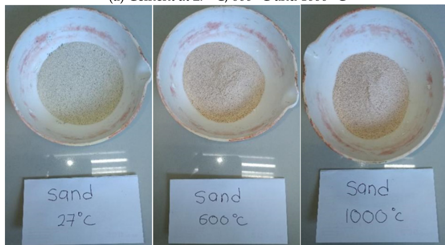
(b) Sand aggregate at 27 °C, 600 °C and 1000 °C
