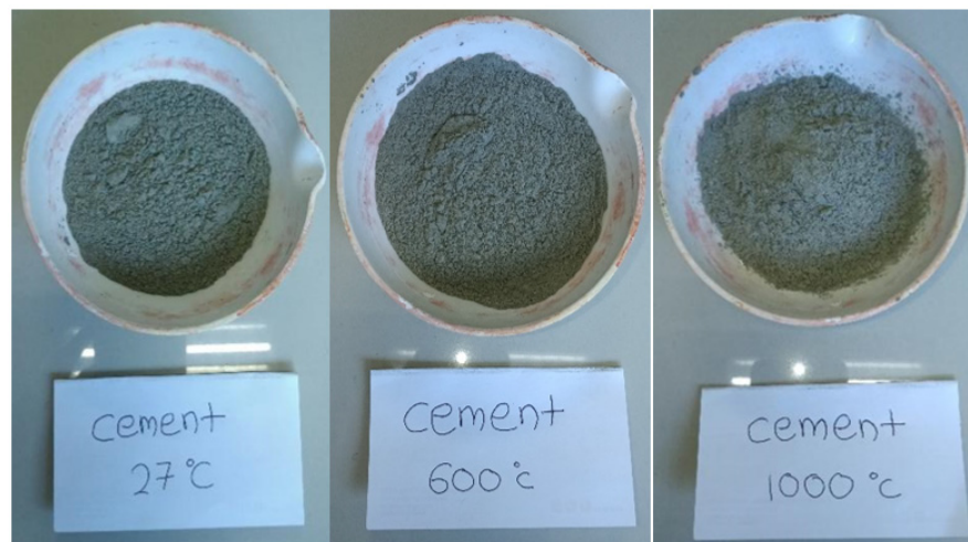
(a) Cement at 27 °C, 600 °C and 1000 °C
