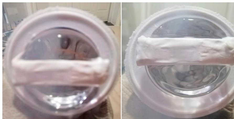
**Figure 7.** The white taped photodetector (MPPC with base board) coupled to the solid argon. The photodetector is put in the solid argon container before solid argon preparation.
