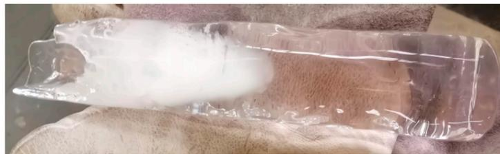
**Figure 4.** Solid argon with an opaque part. The left opaque part is due to insufficient pressure caused by the frozen and blocked pipeline during the preparation.
