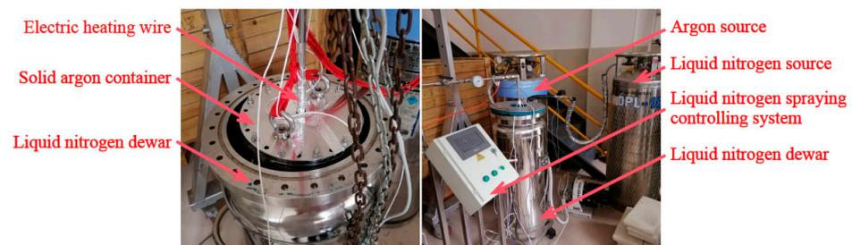
**Figure 3.** Main equipment of our solid argon preparation device.
