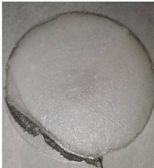
Figure 2. A picture of AlN nanowires on the sapphire.
