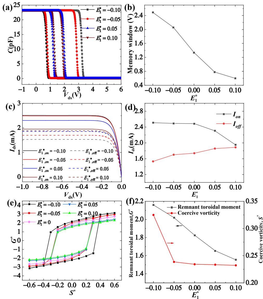
**Figure 2.** Effect of  $E_1^*$  on the ferroelectric topology domain transistors of (a)  $C$ - $V_{ds}$  characteristics of Pt/PtO (20 nm)/Si/SiO<sub>2</sub> structures. (b) Memory window. (c)  $I_{ds}$ - $V_{ds}$  characteristics of Pt/PtO (20 nm)/Si/SiO<sub>2</sub> structures. (d) Open-state current and closed-state current. (e)  $G^*$ - $S^*$ . (f) Coercive vorticity and remnant toroidal moment. The superscript \* indicates the corresponding dimensionless posterior parameter.
