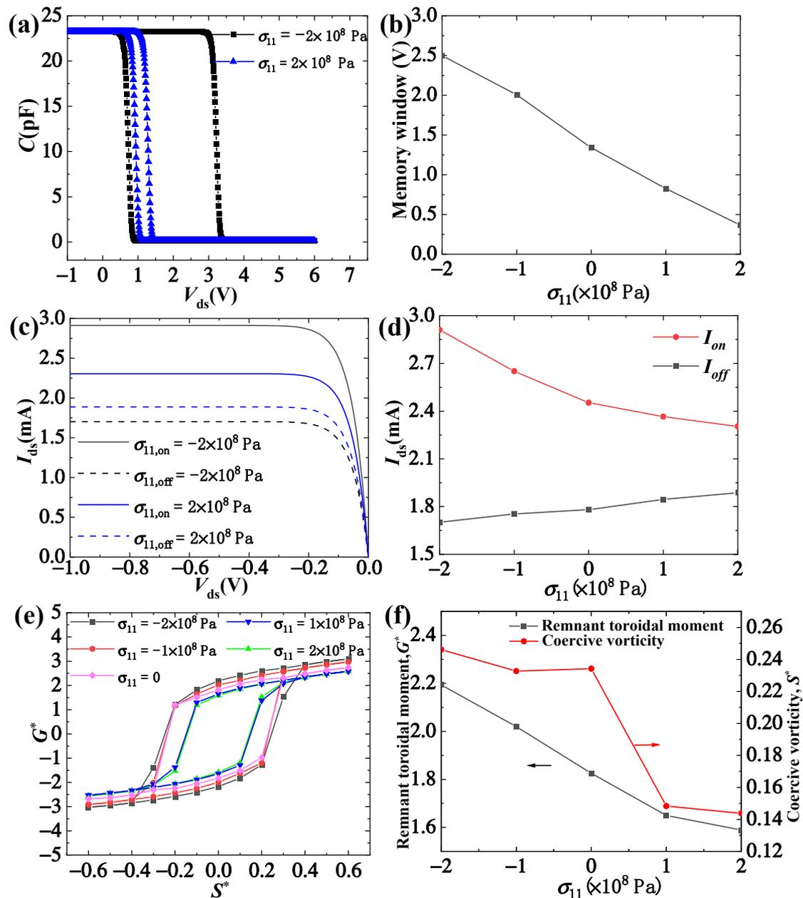
**Figure 3.** Effect of stress on ferroelectric topology domain transistors of (a)  $C$ - $V_{ds}$  characteristics of Pt/PtO (20 nm)/Si/SiO<sub>2</sub> structures. (b) Memory window. (c)  $I_{ds}$ - $V_{ds}$  characteristics of Pt/PtO (20 nm)/Si/SiO<sub>2</sub> structures. (d) Open-state current and closed-state current. (e)  $G^*$ - $S^*$ . (f) Coercive vorticity and remnant toroidal moment. The superscript \* indicates the corresponding dimensionless posterior parameter.
