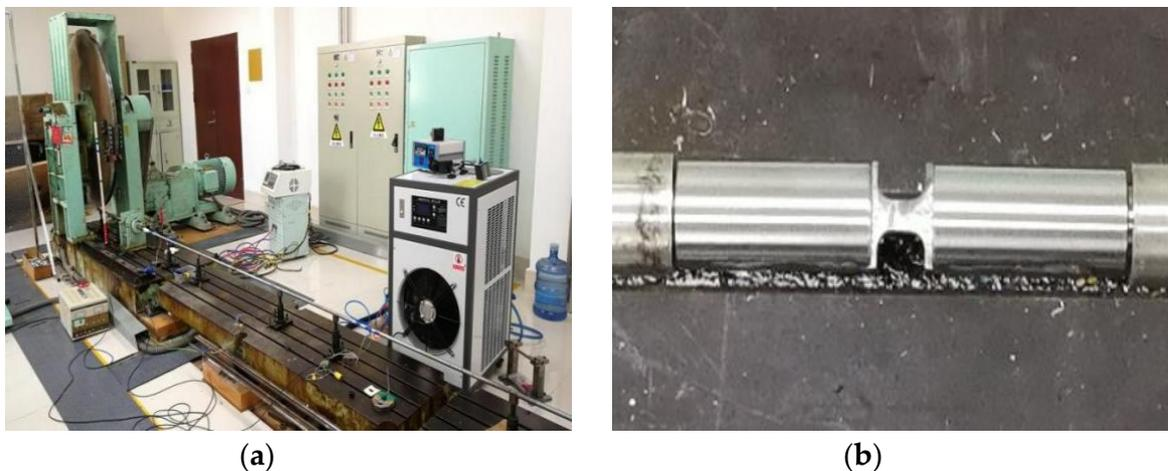
**Figure 4.** Photographs of Hopkinson tension bar and specimen in this study: (a) rotating disk Hopkinson bar; (b) steel specimens.
