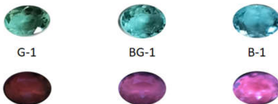
Figure 3. G-1, BG-1, and B-1 apatite fluorescence phenomena. Color under D65 (first row); Color observed in DiamondView fluorescence (second row).
