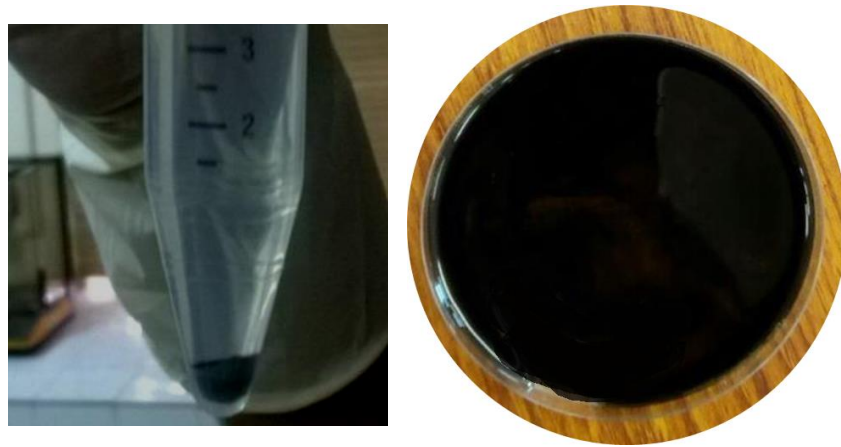
Figure 3. Ag-NPs after centrifugations (left). Silver nanoparticle ink dispersed in ethylene glycol (right).
