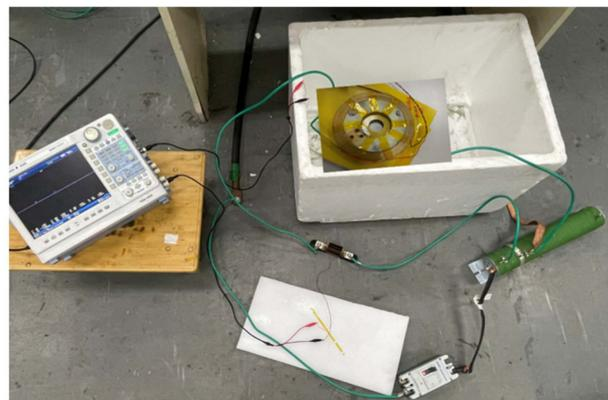
Figure 1. Experiment platform for discharging tests of the HTS coil.
