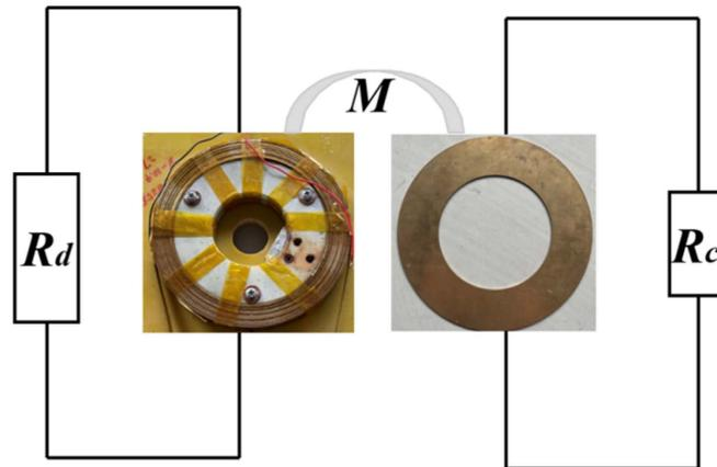
**Figure 2.** Experimental schematic diagram for discharging tests of the HTS coil.
