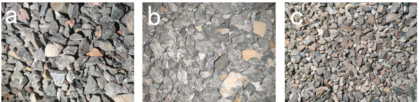
Figure 8. Three kinds of RA with different qualities; (a) SC-RA; (b) OP-RA; (c) DP-RA.
