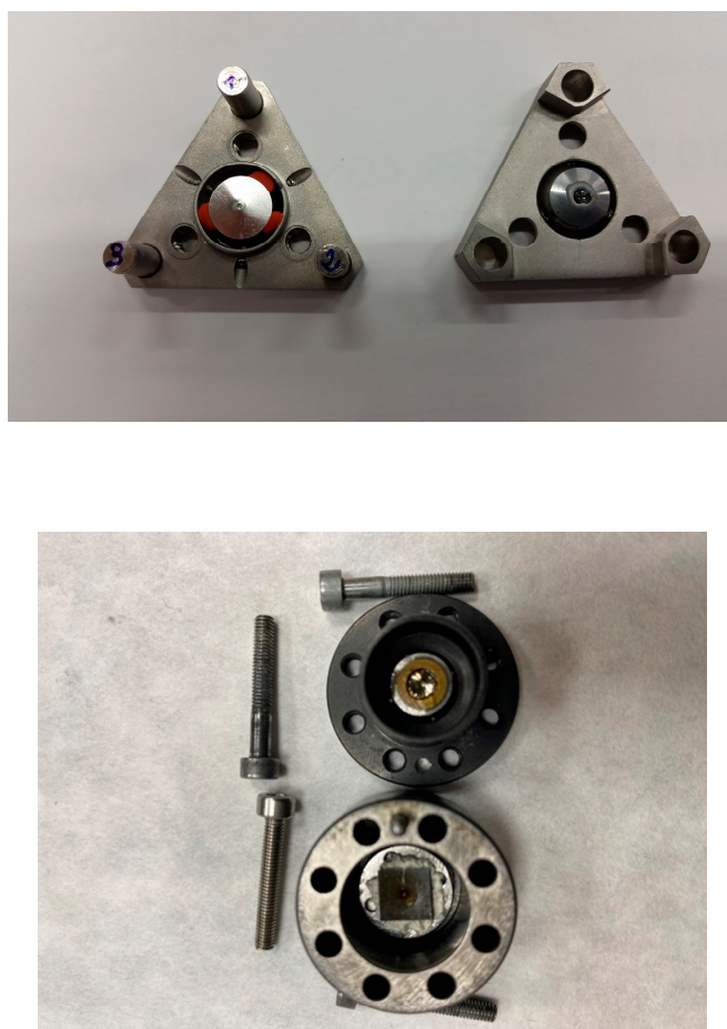
Figure S2. Bragg-Mini DAC (Almax EasyLab company) with 500 \mu m diameter in the culets of diamonds (top). Paderborn Mini DAC with 400 \mu m diameter in the culets of diamonds (bottom)
