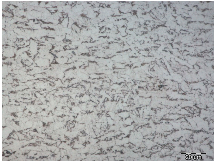
Figure 6. Microstructures of the base metal (with a magnification of 1000).
