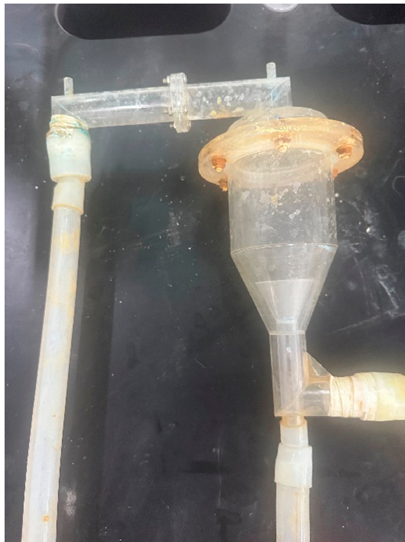
Figure 15. Dynamic liquid phase crystal growth device.
