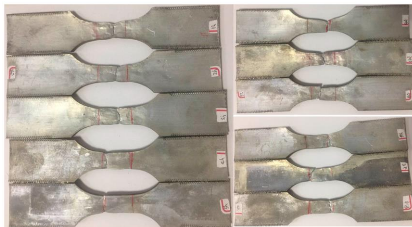
Figure 15. Fracture diagrams of the 6061 aluminum alloy specimen after secondary heat treatment.
