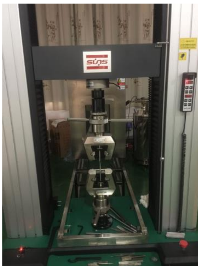
Figure 2. Test loading device.
