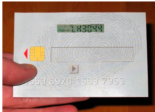
Figure 6. Color online. Prototype of ORW e-paper technology for a smart card.
