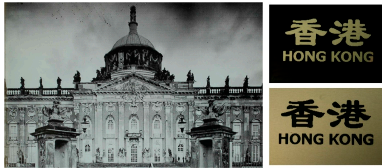
Figure 4. ORW e-paper image showing grayscale. Left: Image with a resolution of 140 ppi. Right: two images of ORW e-paper with crossed and parallel polarizers.
