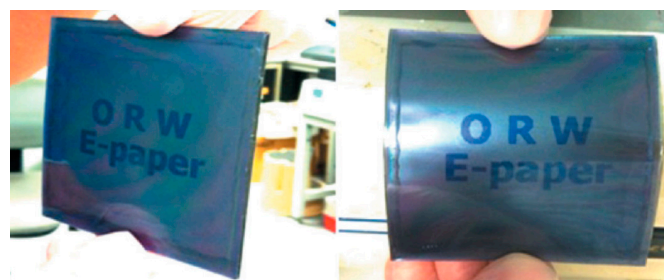
Figure 3. Sample images showing flexibility of ORW e-paper.
