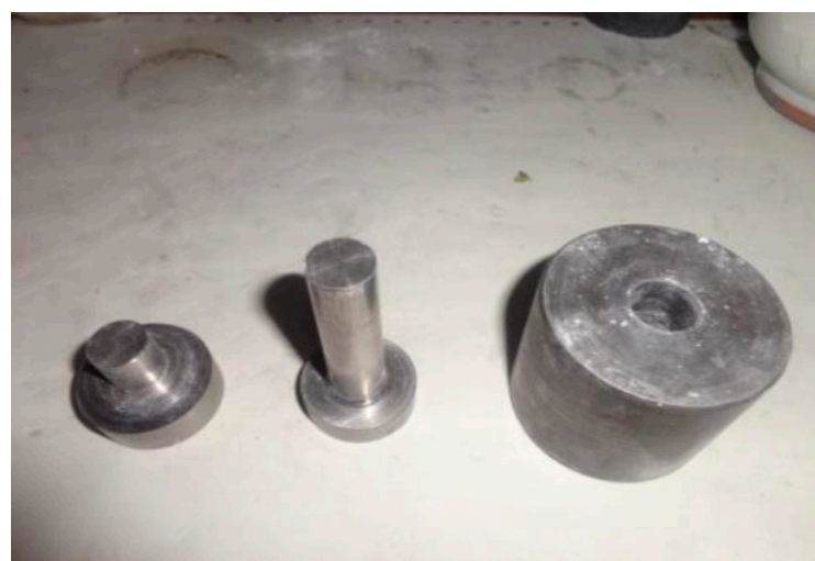
Figure 1. Die assembly used for making compact samples with the help of hydraulic press. The diameter of samples to be prepared is 20 mm and the thickness is 4 mm.
