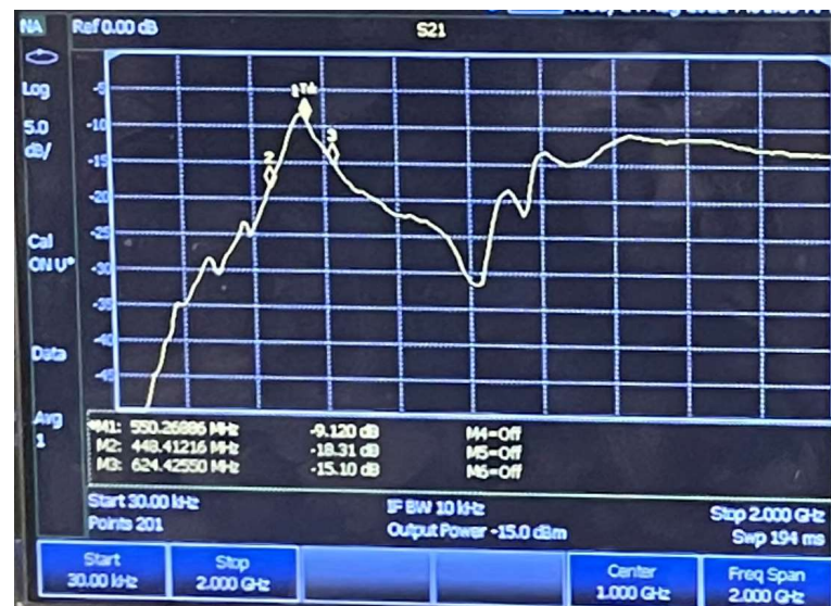
Figure 3. S 21 measurement of the BST based SAW sensor with Indium doped SnO 2 with a 2.5 μm of finger width and spacing of the IDT structures. The fundamental resonance was around 550 MHz. Higher order resonances can also be seen.
