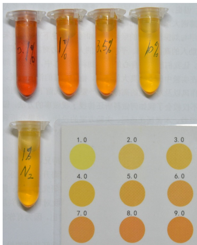
Figure 4. Dissolved oxygen content (mg/L) of NaCl solution with different Cl^- concentrations.
