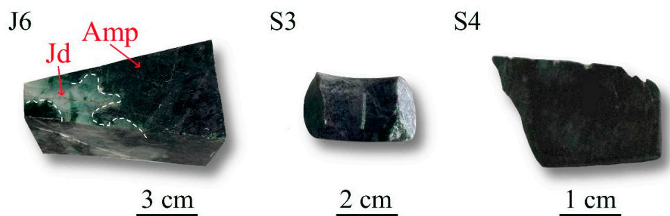
Figure 2. Photos of amphibolite samples with black chromite and green kosmochlor.
