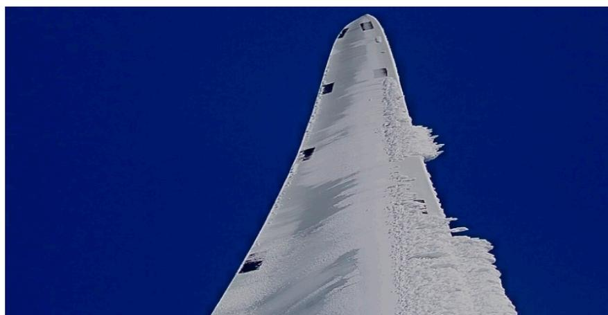
**Figure 2.** A blade of wind turbine in icy conditions [provided by Nergica-June 2020].
