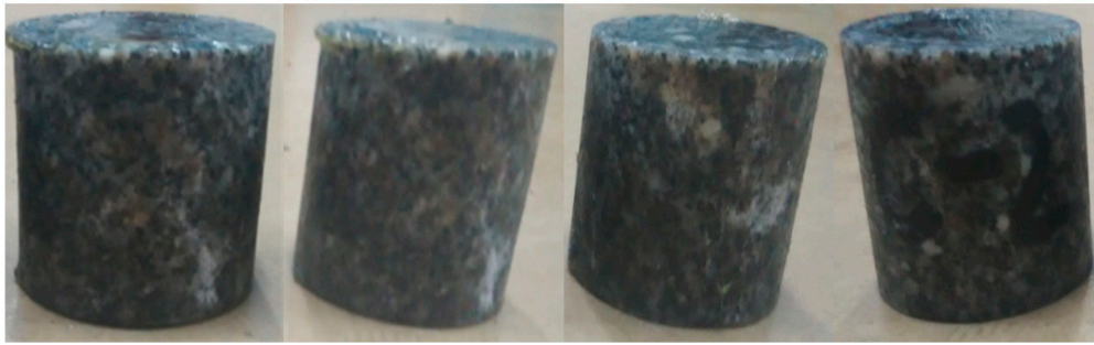
Figure 6. Rock samples after the cycle dynamic impact test.
