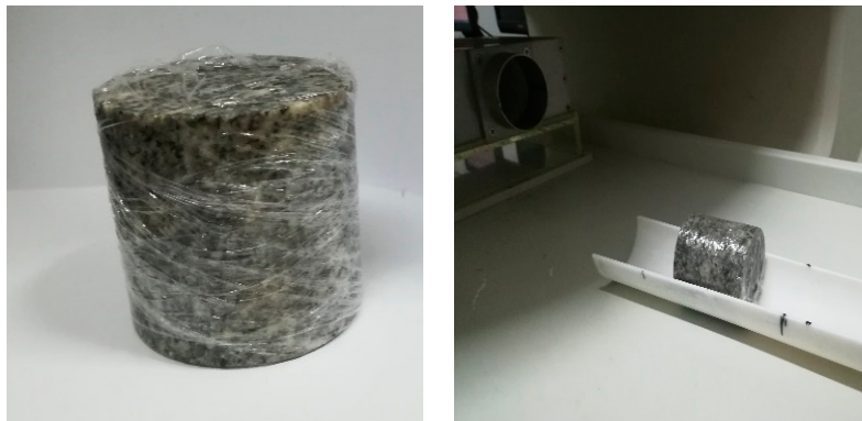
Figure 2. Preparation of rock samples before testing.
