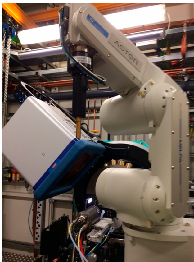
Figure 2. The ACTOR robot mounting device in place on beamline I19, DLS; the Pilatus detector, part of the goniometer, and the Cryostream sample cooler can be seen in the background.
