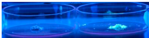
Figure 11. The photographic picture exposed at 365 nm under an ultraviolet lamp ( H_2L ligand, (left); complex 1 , (right)).
