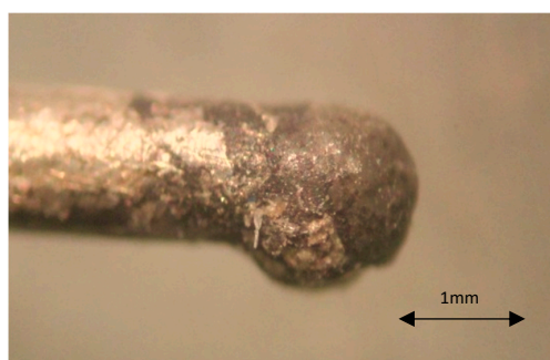
Figure 6. Magnified image of a damaged K-type thermocouple tip (source: IHPP PAS).
