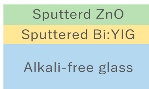
Figure 2. Representation of a cross-section of a fabricated ZnO/bismuth-substituted yttrium iron garnet (Bi:YIG) bilayer.
