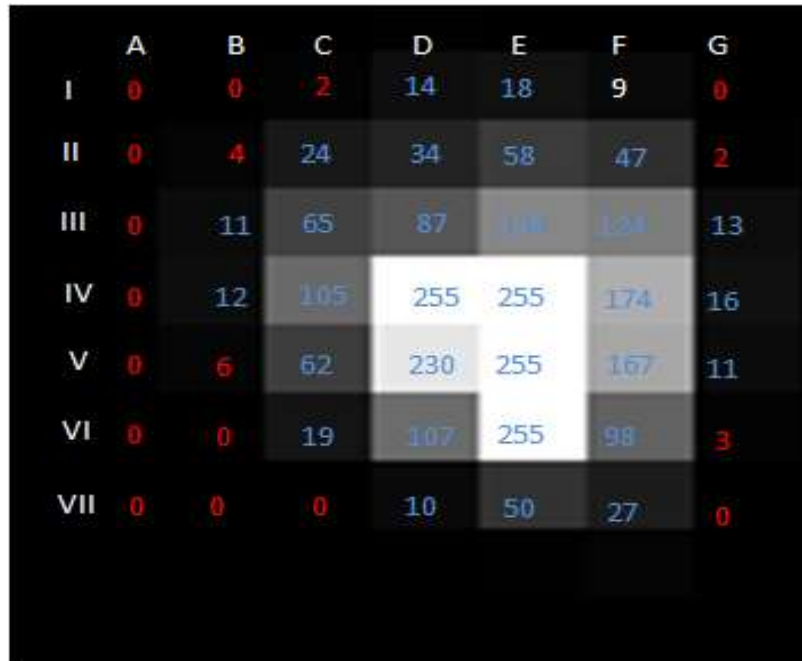
Figure 2. Grayscale variations of a protrusive defect with respect to the threshold.
