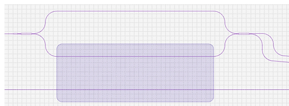
Figure 2. The tested MZI structure with multimode interference (MMI) in and out coupling. The LC is located in the dashed area. The straight line at the bottom is another waveguide that is not employed in this setup.
