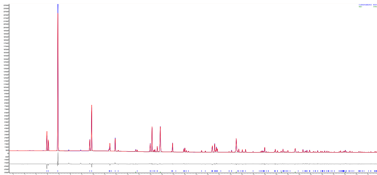
Figure S22. Rietveld plot for refinement of r -Co(MeOH) 6 B 12 H 12 at T= 62 °C. SNBL, \lambda = 0.77936 \text{ \AA} , \chi^2 = 665 , R_{wp} (bgr. corrected) = 0.10, R_{Bragg} = 0.04 .
