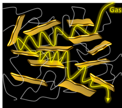
Scheme 2. Barrier to permeation imposed by nanoparticles embedded in a polymeric matrix.
