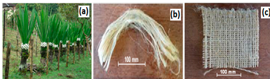
Figure 1. Plantation of fique ( Furcraea andina ) in Colombia (a), bundle of fique fibers (b), and as-received piece of fique fabric (c).
